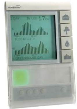
ecoMeter: A consumer energy display device being offered by Cellnet+Hunt
